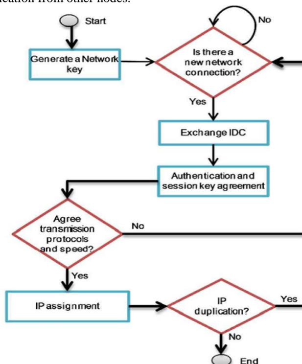
Figure 3: Procedure for joining a new node
