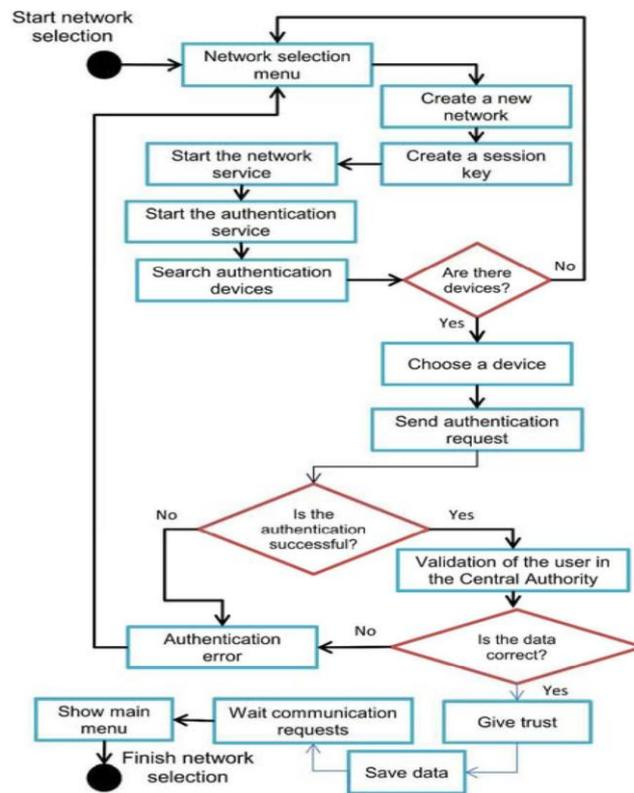
Figure 5: Procedure for new network creation
